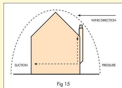
As this condition usually occurs only with the wind in a certain quarter, the situation of the chimney in relation to the roof will indicate the cause of trouble; furthermore, smokiness normally occurs only when there are openings (doors or windows) on the low-pressure side but not on the high-pressure side.
