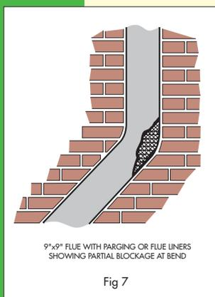
*Another method of checking a flue for obstructions is to lower a 'coring ball' on the end of a rope down the flue. The coring ball of concrete or metal, which should be of such a size that it has not more than 25mm (1in) clearance in the flue, will determine the exact position of the blockage if a knot is tied in the rope when the ball gets stopped, and may even dislodge it.*
